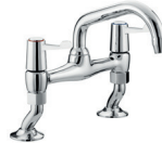
Pillar Bridge Sink Mixer Height 230mm Spout projection 210mm 3" Levers Dual flow prevents hot water entering the mains supply
